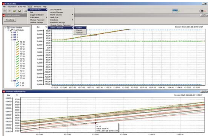
Validation system with 64 temperature channels and 2 pressure channels.
