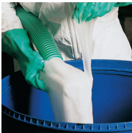
CMC: virtually "sausage like" extrusion
