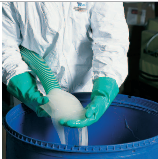
Xanthan: virtually "sausage like" extrusion
