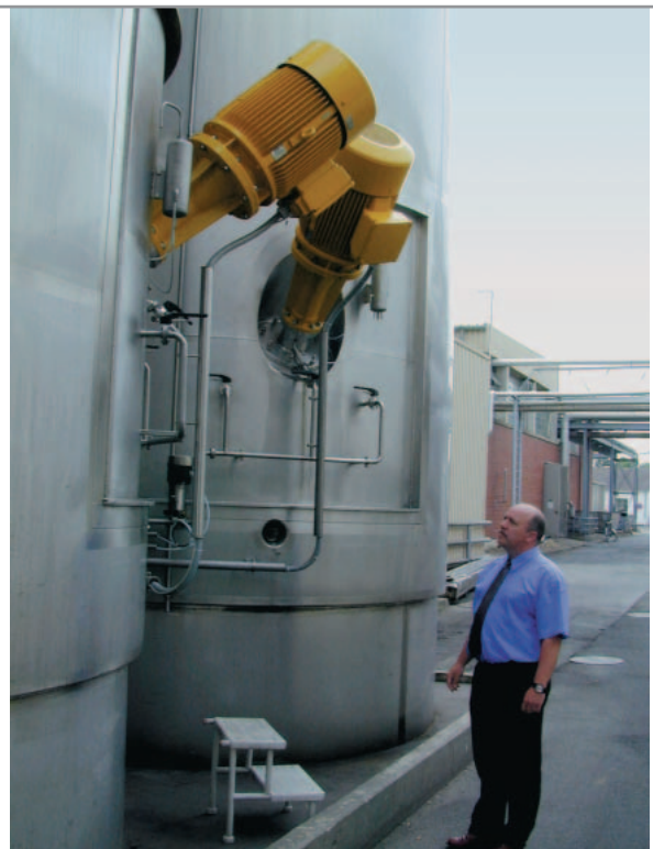
YTRON -Y in Side Entry Tank-flange execution below Liquid Level Application: Fermented Milk for Fromage Frais Production (100.000 litres capacity)
