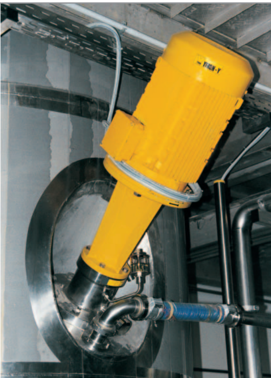
YTRON-Y in Tank-flange Construction, installed in a Closed Vessel Application: Shampoos and Shower Gel and similar Toiletry Products
