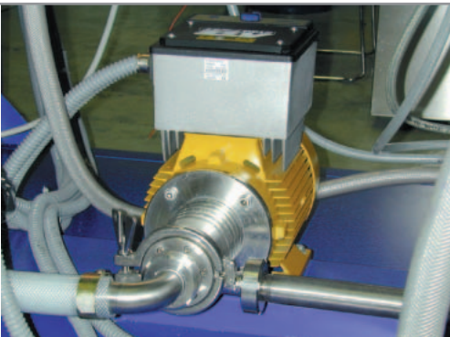
YTRON-Z with integrated frequency control Application: Continuous production of base thickeners in the Textile Printing Industry
